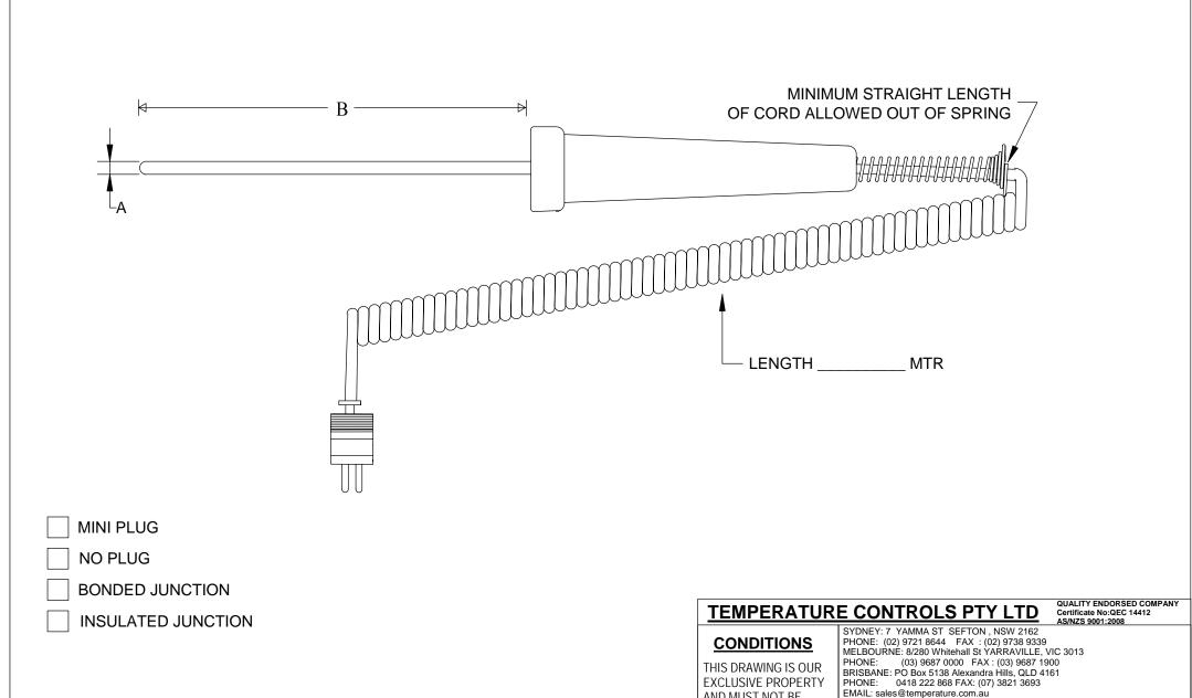
THERMOCOUPLE HAND HELD IMMERSION PROBE
